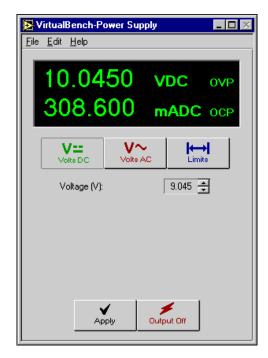
Figure 7-3. Front Panel with Volts DC Button Selected
